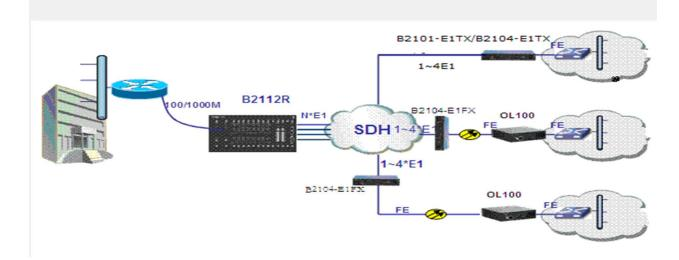
When end-user is near to SDH transmission equipment room, B2101-E1TX/B2104-E1TX can be used to provide 1 channel TX to 4E1 conversion, offering 4E1 aggregation with any combination over B2104-E1TX, 2~8M access bandwidth is available. Otherwise, OL100 MC and B2104-E1FX can be used in pair, convert the Ethernet into 1~4\*E1 then access to transmission network.
