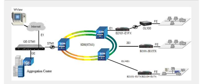
In user's branch node, versatile interface converters can be used based on specific access requirements including B2101-E1TX, B2104-E1TX (or B2104-E1FX+OL100), B2101-2E32TX, etc., realizing E1/E3 service access. In aggregation center, GE-STM1 product can also be inband managed via E1 channel or out-of-band network management port.
