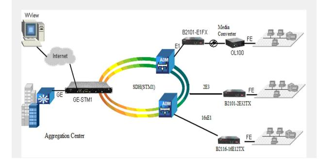
GE-STM1 product can be used in ring topology. In this way, GE-STM1 works as the central node of SDH STM-1 ring, offering 1-channel GE data uplink.
